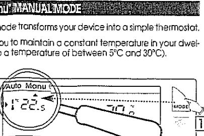
1 Press the "MODE" button to position the pointer under "Manu".
