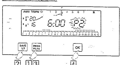
① Press the PROG P1-P4 button to go into programming mode. The N° of the programme assigned to the day flashes on the right-hand side of the display panel.
