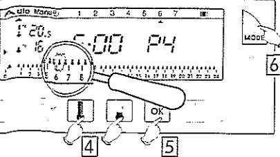
4 Press the button several times to obtain 0:00. The time display advances by 30 minutes for each short press. Continuous pressing accelerates the time run-off.
